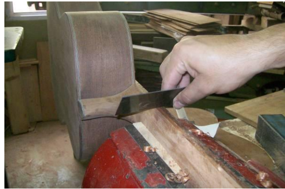
Figure 11 - The heel where the neck is joined with the body of the guitar (top).
