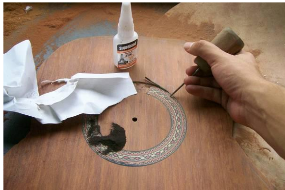
Figure 9 - Guitar rosette. A router was used to create the trench for installing the rosette. A black colored wood glue was used to match the dark tones of the wood. Any gaps were filled in with small pieces of wood and carved into place (bottom right).
