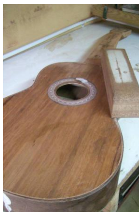
Figure 10 - Template for the spines (left) which are directly under the front soundboard (right).
