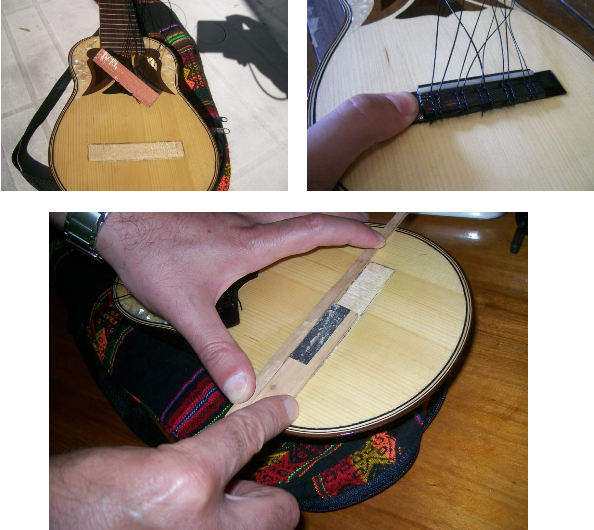
Figure 24 - Space where bridge was attached (left). Sanding away the previous adhesive (bottom). Replacing the bridge (right).
