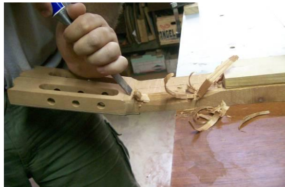
Figure 12 - Drilling holes for the tuners (left). Filing my design onto the head (top right). Carving the neck (bottom right).
