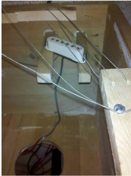
Figure 20 - Guitar pickup positioned behind the "snare" strings (left). 1/2" jack on the back of cajon (right).
