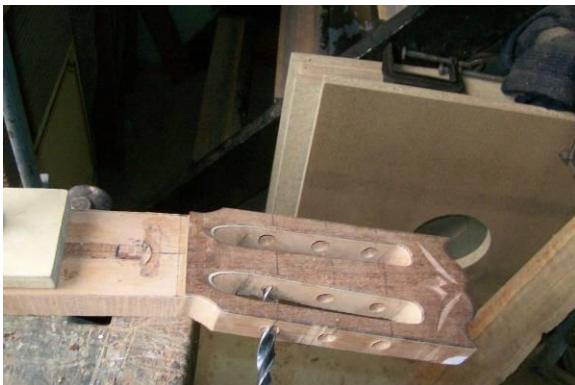
Figure 12 - Drilling holes for the tuners (left). Filing my design onto the head (top right). Carving the neck (bottom right).
