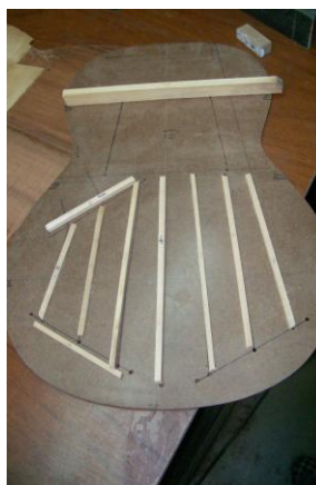
Figure 10 - Template for the spines (left) which are directly under the front soundboard (right).
