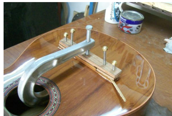
Figure 16 - Bridge (top left). Setting the glue for the frets (top right). Installing the bridge (bottom).
