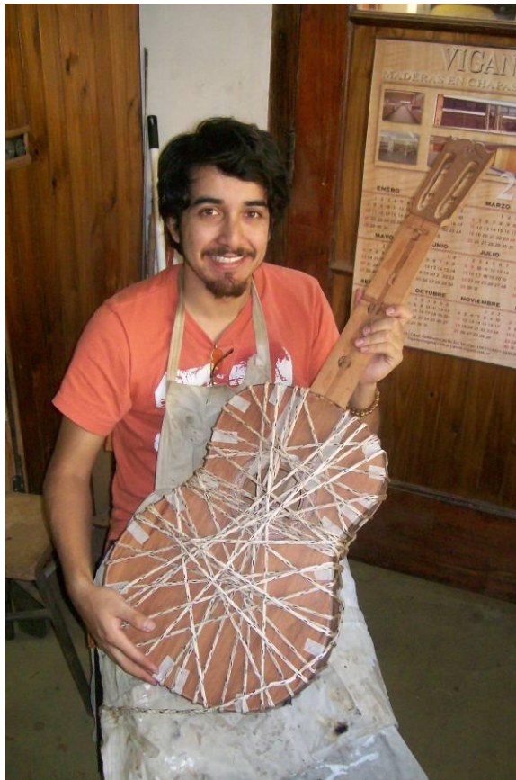
Figure 14 - Gluing the sides of the guitar. To hold them in place I wrapped the entire body with string.
