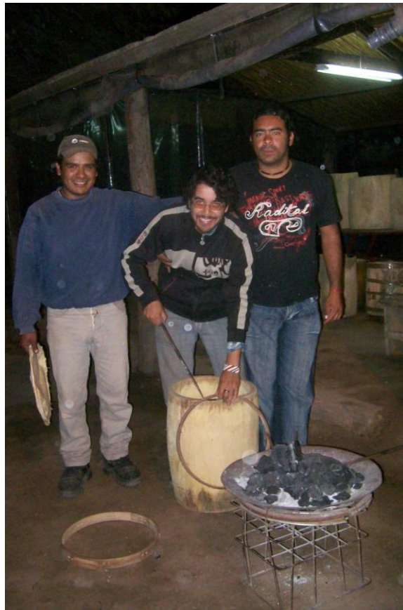
Figure 23 - Bass Drum. Burning a hole in the rim for tightening the cowhide rope.
