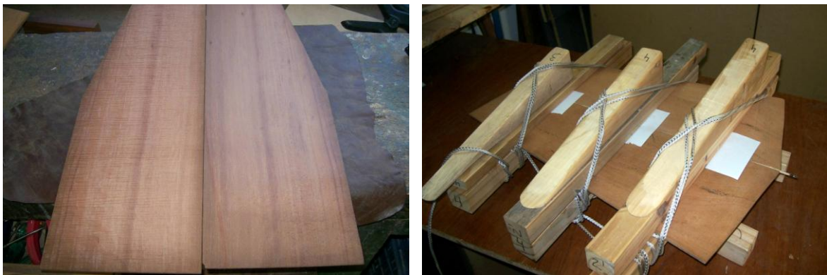
Figure 7 - Beginnings of my classical guitar. The front and back of the body are made from two pieces joined in a press made of wedges and string (right).
