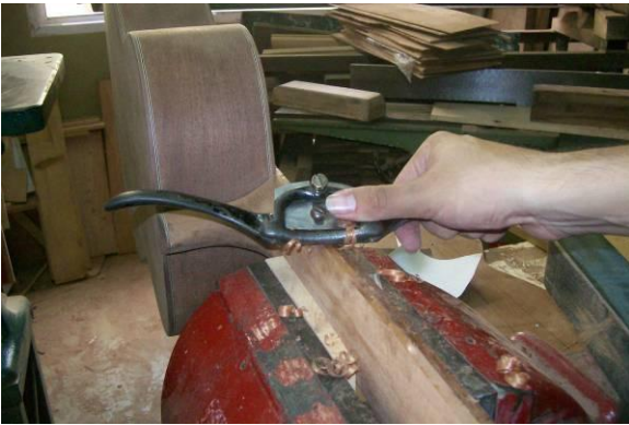
Figure 11 - The heel where the neck is joined with the body of the guitar (top).
