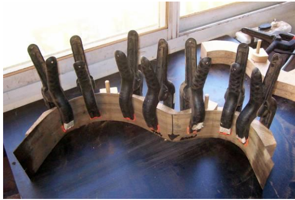
Figure 13 - Jig used to form the sides of the guitar.
