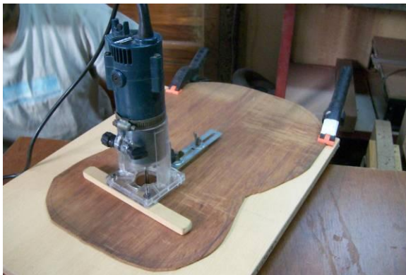
Figure 9 - Guitar rosette. A router was used to create the trench for installing the rosette. A black colored wood glue was used to match the dark tones of the wood. Any gaps were filled in with small pieces of wood and carved into place (bottom right).
